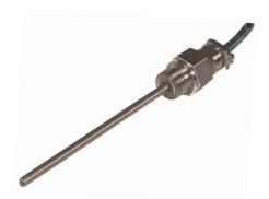
Platinum resistance temperature sensor built into steel tube V4A, 1/2 inch, suitable for installation in pipes. Thermal response time T0,9 in the air 255 s, in water 45 s. Connection flat plug 2,8 mm, Gasket IP55, clamping diameter 8-12 mm, cable connection max 100 °C Suitable for transmission in 2- or 3-wire technique
