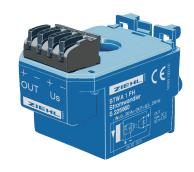
Part number: S225560 The STWA1FH provides a frequency output with 0.5...20 Hz which corresponds to a current flow of AC 0 - 20 A through the transformer. Multiple loops of the conductor through the transformer reduce the current range correspondingly (e.g. with fourfold looping-through 0 - 5 A correspond to 0.5...20 Hz).
