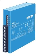
Part number: V223267 The level monitor NS43 regulates the level of liquid in a container between 2 electrodes. In the normal operation the level of the liquid is situated between the electrodes E2 and E3. The relay K2 tightens, if the level E3 is achieved and drops, if E2 is fallen below. Over the output contacts (1 change-over switch) a pump or a valve can be controlled depending upon case of application and so the level be
