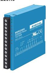
Part number: T221958 AC/DC 24-240 V The MSR220K6 monitors up to 6 PTC-reseitor sets with up to 6 PTCs each at the same time. If a temperature rise occurs in one set, the output relay releases and LEDs show the overheated sensor.
